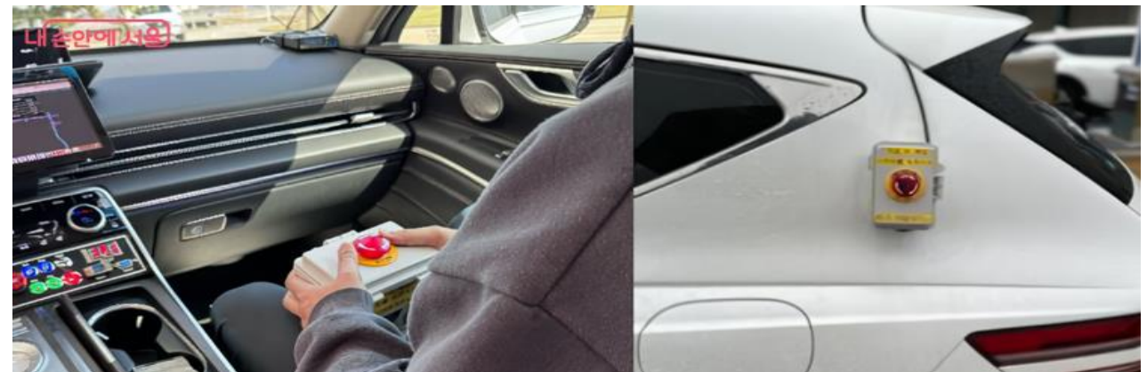
Emergency Stop Switches Installed both inside and outside the Phase 4 autonomous vehicles in Sangam-dong ©Rideflux
